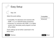
The "Compatible" setting configures audio output in a way that is generally compatible with all types of equipment and content. If you connect the player to a television directly, or to a receiver with an HDMI 1.1/1.2 or optical/coaxial input, selecting the "Compatible" setting is recommended. When menu click sound and Secondary Audio Program are presented in the content, those will be mixed into the audio output.
